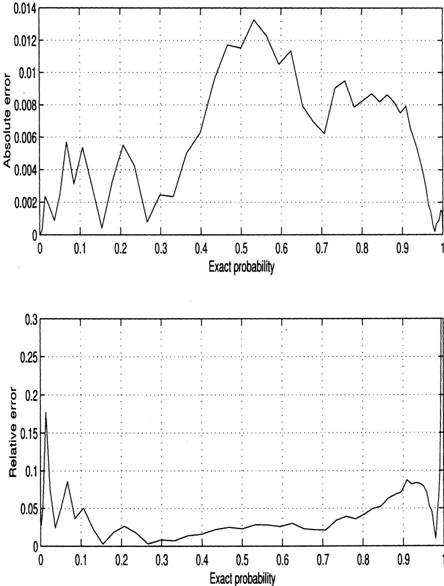
Figure 2. Saddlepoint approximation for the distribution of the resultant length under the WN distribution,  $\mu = 0$ ,  $\sigma^2 = 4$ ,  $n = 6$ . Upper figure: absolute error  $|P_E - P_S|$ . Lower figure: absolute relative error  $|P_E - P_S| / \min\{P_E, (1 - P_E)\}$ .  $P_E$ : exact distribution obtained by  $10^6$  simulations.  $P_S$ : saddlepoint approximation to the distribution. The abscissae are the exact probabilities.
